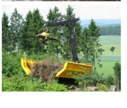
behind the forwarder. Most of the time is lost on loading, so it is of great importance that the harvester places the cut trees in an optimal position for collection.
